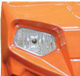
Low- and high-beam head lights
