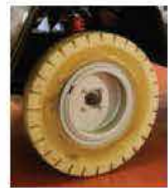
No-marking + foam filled tyres
