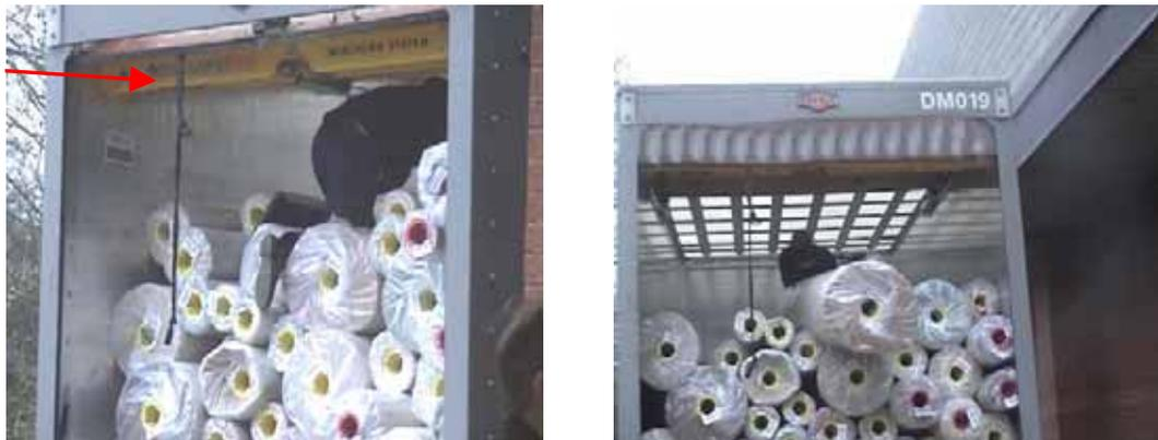
**Figure 10. Example of an employee climbing into the back of the lorry and manually pushing the carpet rolls out rather than using the 'Carpet Tug'.**
