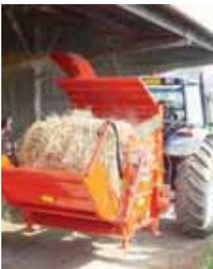
**Figure 7** Tractor-mounted straw chopper for spreading fresh bedding
