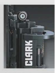
Upright & Carriage Sealed, canted rollers minimize deflection and side play in both upright and carriage. Six carriage rollers and two side thrust rollers reduce roller contact stress to extend upright life. Hydraulic cushioning valves provide silent staging of the rails to reduce shock during both lifting and lowering.
