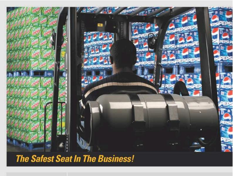
Safety seat More than 160,000 safety seats have been installed on CLARK trucks. CLARK is the innovator of the safety seat and today our offer the best in safety features. Side wings and a standard seat belt, with retractors that won't tighten during use, are standard. The durable molded seat is adjustable horizontally up to six inches. Optional seats with semi-suspension, and'or durable fabric covering are also available.
