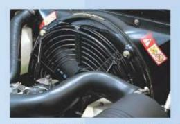
Cooling system The open-core, plate-fin, cross-flow radiator design with integral transmission oil cooler has wide fin for reduced plugging and easy cleaning. A coolant recovery system allows easy fluid level checks and adding coolant without opening the pressurized radiator cap. The 7-blade flexible fan uses a venturi shroud to optimize performance and reduce noise a grille to guard the fan.
