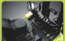
Just simply opening the two-pieced rear hood, assisted by a gas spring, allows quick and easy access to engine, transmission, radiator and air cleaner for daily checks and maintenance.
